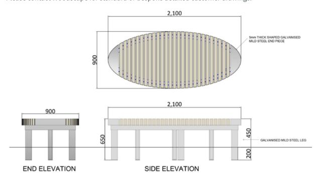
Technical Data: Lime rove Seat with void - 2100mm x 900mm
